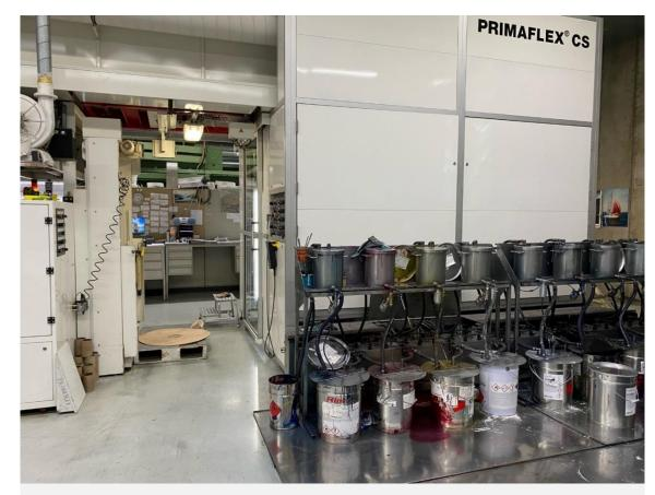
W&H Primaflex CS 8-station with InkSight system integrated in the press as a modular unit
