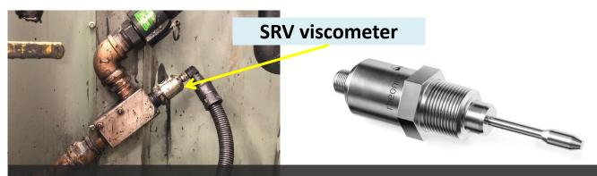
Inline ink viscosity monitoring by Rheonics SRV viscometer
